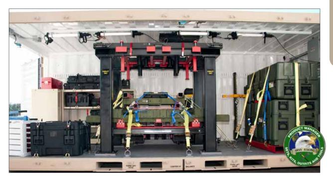
The Stryker Special Tools Set System is a set of selected tools and equipment used to maintain the Stryker combat vehicle system on or near the battlefield. The tools and equipment are placed in a rapidly deployable tactical shipping container and storage system, ISO type 1C (8 ft high, 8 ft wide, 20 ft long). Altogether the container provides weather tight security for when the container is on board a ship and other environments.
